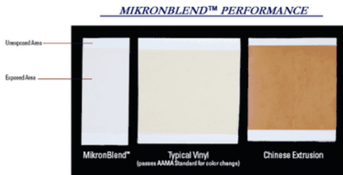
Actual, unaltered photo of samples after 1 year equivalent UV accelerated weathering Xenon-Arc.
